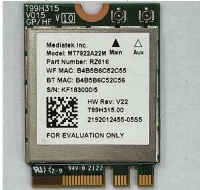
(17) EUT Photo WLAN (Mediatek/MT7922A22M)
