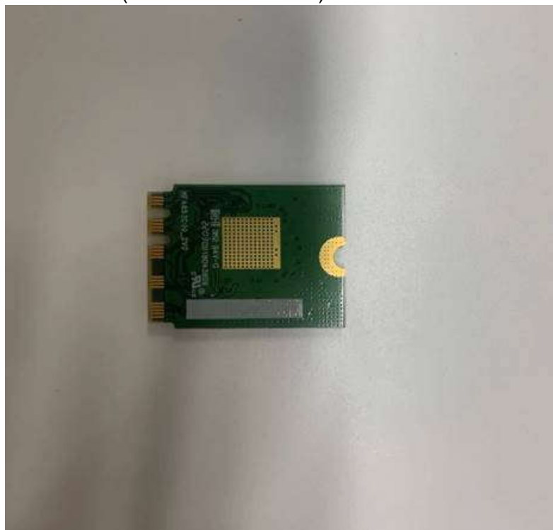
(21) EUT Photo WLAN (Realtek/RTL8852CE)
