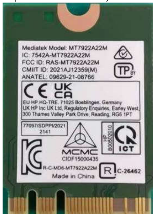
(18) EUT Photo WLAN (Mediatek/MT7922A22M)
