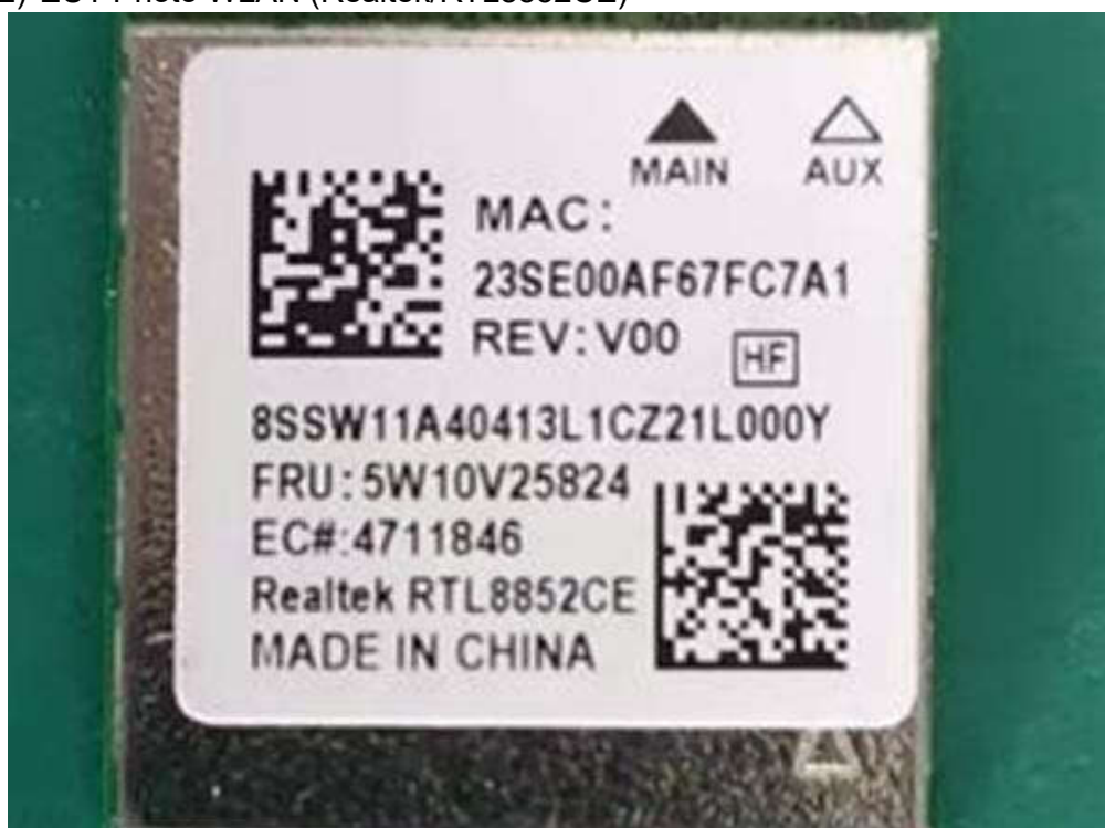
(22) EUT Photo WLAN (Realtek/RTL8852CE)
